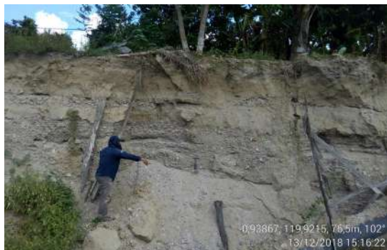
Figure 4.3.20. The outcrop of the Petobo landslide crown showing alternating layers of gravel - pebbles (sediment gravity flow products) and sand (sand bedforms products) (Sumber: Buana, 2018).
