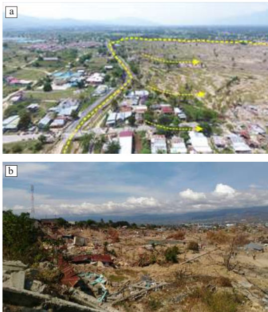
Figure 1.1. Flow liquefaction occurring in Petobo (a) and Balaroa (b) as a result of the Palu earthquake in 2018.
