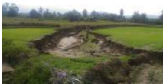
Figure 1.3. Lateral spreading observed in the Jono Oge area.
