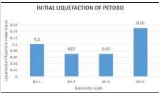
Figure 4.3.27. Initial liquefaction at locations BH-1, BH-4, BH-2, and BH-5 in Petobo.
